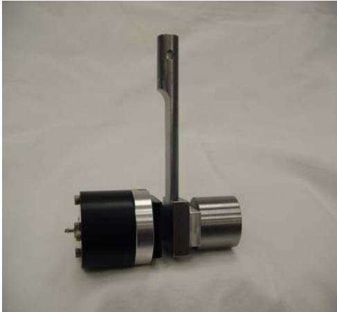
MT Series Air Grip for Tissue with 1 inch x 1 inch Rubberized Inserts installed.
