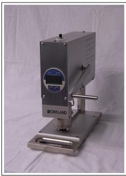
The Model GP-175 MicroGauge Thickness Tester.
